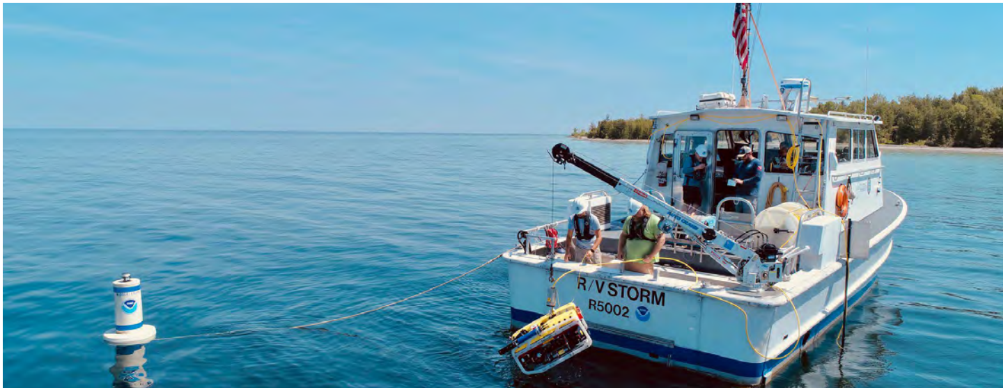
Deploying an ROV to install flow meters at the Middle Island Sinkhole in Lake Huron. (Photo Credit: David J Ruck/Great Lakes Outreach Media)
