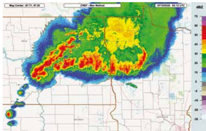
Composite reflectivity field at 0012 UTC July 17, 2020 over the north-central United States produced by the Multi-Radar Multi-Sensor (MRMS) system using code hosted on the public cloud.
