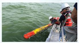
For the third year in a row, NOAA is using Environmental Sample Processors designed by the Monterey Bay Aquarium Research Institute and mounted on a UUV to study potentially toxic algal blooms in Lake Erie in collaboration with NOAA's Great Lakes Environmental Research Laboratory.
