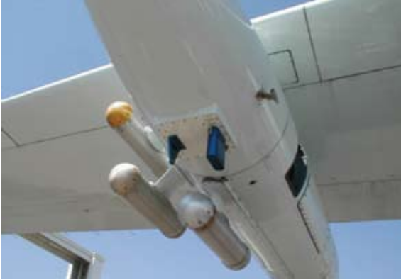
Figure 8.3. An aircraft-based water vapor sensor was successfully field tested in 2005-2006 on commercial aircraft. Results of the test were presented at the American Meteorological Society Conference in 2006. Increased observations from sensors deployed using aircraft of opportunity will support improvements to numerical models used in NOAA products and services
