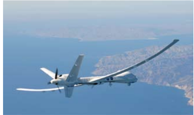
Figure 8.2. In FY 2006, NOAA, NASA, and a private sector firm successfully evaluated the potential for Unmanned Aerial Systems (UAS) to meet NOAA operational needs. The Altair UAS was used to carry a variety of sensors including the Digital Camera System (DCS) and Electro-Optical Infrared (EO/IR) Sensor to demonstrate how operational needs of NOAA could be met in future UAS flights. The DCS was used in shoreline mapping and in along-shore/inland feature characterization for habitat mapping/ ecosystem monitoring. The EO/IR system was used for fisheries surveillance and marine mammal surveys.
