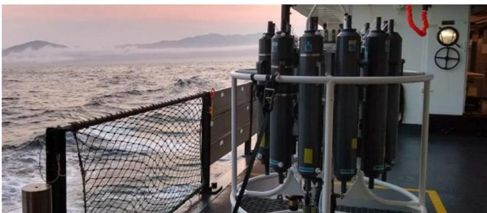
A conductivity, temperature, and depth instrument is shown on deck. Scientists gathered water samples at multiple depths across 186 locations off the West Coast during hake surveys on the NOAA Ship *Bell M. Shimada* in 2019. Photo credit: NOAA Fisheries
