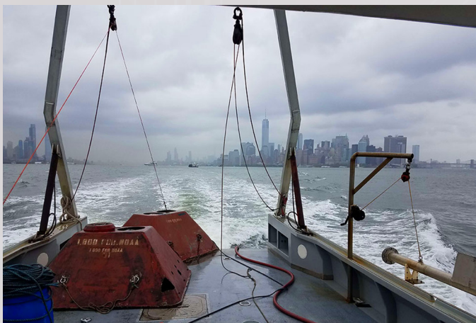
NOAA oceanographers deploy sensors like these in the water to measure tidal currents for a period of time and then return to collect them. The two sensors pictured here were recovered from the Hudson River, just off the coast of Lower Manhattan in New York. NOAA NOS, Center for Operational Oceanographic Products and Services
