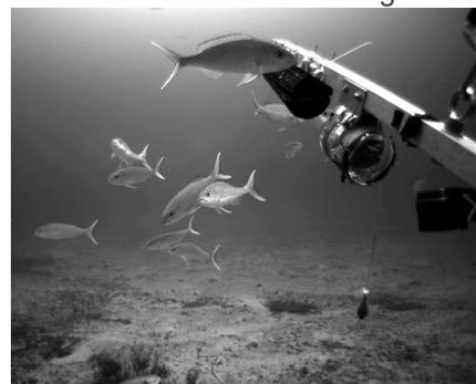
Figure 4. The Modular Optical Underwater Survey System (MOUSS) is one of several technologies NOAA Fisheries is using to study Hawai'i's fish populations.
