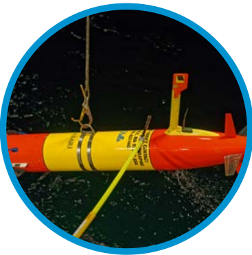
Researchers at the NEFSC and Woods Hole Oceanographic Institution retrieve an autonomous underwater vehicle equipped with cameras surveying sea scallops during a 2024 research cruise. Credit: Dvora Hart
